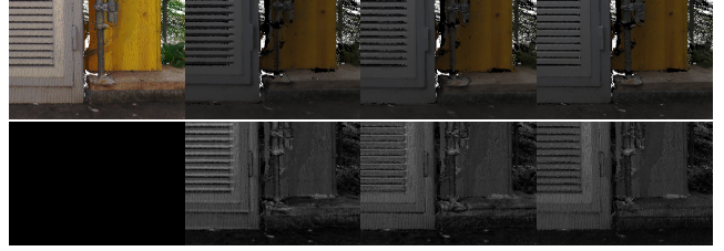
Figure 4. Two examples of laser scan renderings colored by differently aligned images. Top row, from left to right: Original laser scan colors, initial alignment, 7-DoF ICP alignment, our alignment. Bottom row: Difference of each image to the laser scan image. Note that the different lighting causes a significant color difference.
