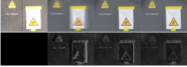
Figure 4. Two examples of laser scan renderings colored by differently aligned images. Top row, from left to right: Original laser scan colors, initial alignment, 7-DoF ICP alignment, our alignment. Bottom row: Difference of each image to the laser scan image. Note that the different lighting causes a significant color difference.
